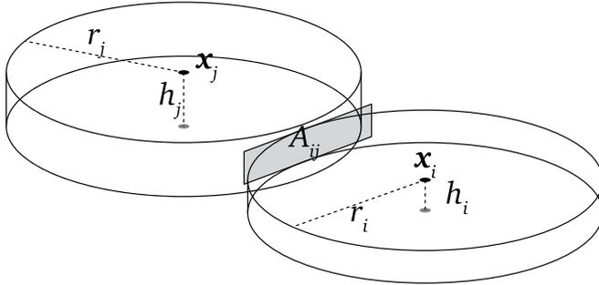
b) Post-failure contact geometry
